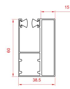
**HD60 Guide** Approved fixings and installation instructions provided with the shutter for fixing to brick, block, aluminium and steel.
